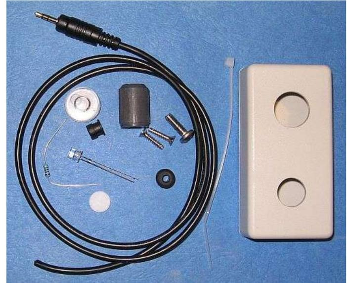
The *Institute for Earth Science Research and Education* has sold hundreds of pyranometers in kit form (US\$20) and assembled and calibrated. Kit-built pyranometers must be calibrated against a reliable standard or by using a clear-sky model over time. Once calibrated properly, these instruments will produce reliable data for years. The least expensive commercial silicon-based pyranometer costs about US\$200.
